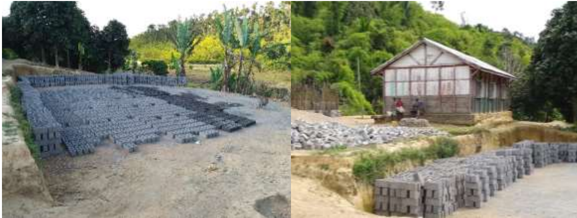
Figure 7 Cement breezeblock production
